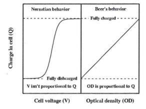
Figure 4: Schematic illustrations of the capacity-monitoring techniques for a battery based on the voltage and optical measurements.
