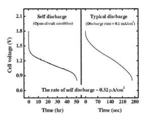
Figure 9: Comparison between self-discharging and typical discharging of a PWECB.
