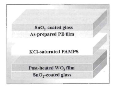
Figure 1: Schematic illustration for assembling a thin-film PWECB.
