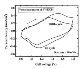
Figure 8: Comparison between the two-electrode voltammograms of the  $1^{st}$  cycle and the  $100^{th}$  cycle for a PWECB
