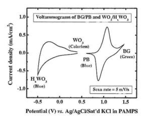
Figure 2: Typical cyclic voltammograms for the BG/PB and  $WO_3/H_xWO_3$  redox couples.
