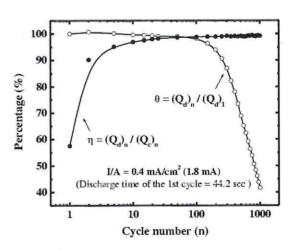
Figure 7: Cycling characteristics of a fresh PWECB, which was charged/discharged between 0.80V and 1.80V 1,000 times.
