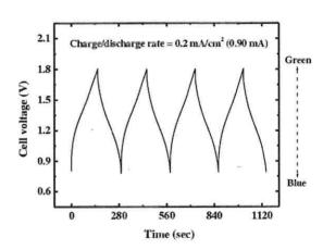
Figure 3: Typical cell voltage for a PWECB charged and discharged at a rate of 0.2 mA/cm<sup>2</sup>.
